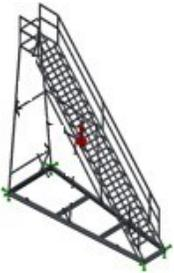
A 3D wireframe model of a staircase. The base of the staircase is fixed to a horizontal plane, indicated by green arrows pointing outwards from the base, representing fixed boundary conditions. | Tipo: Geometría fija al piso en las ruedas |
