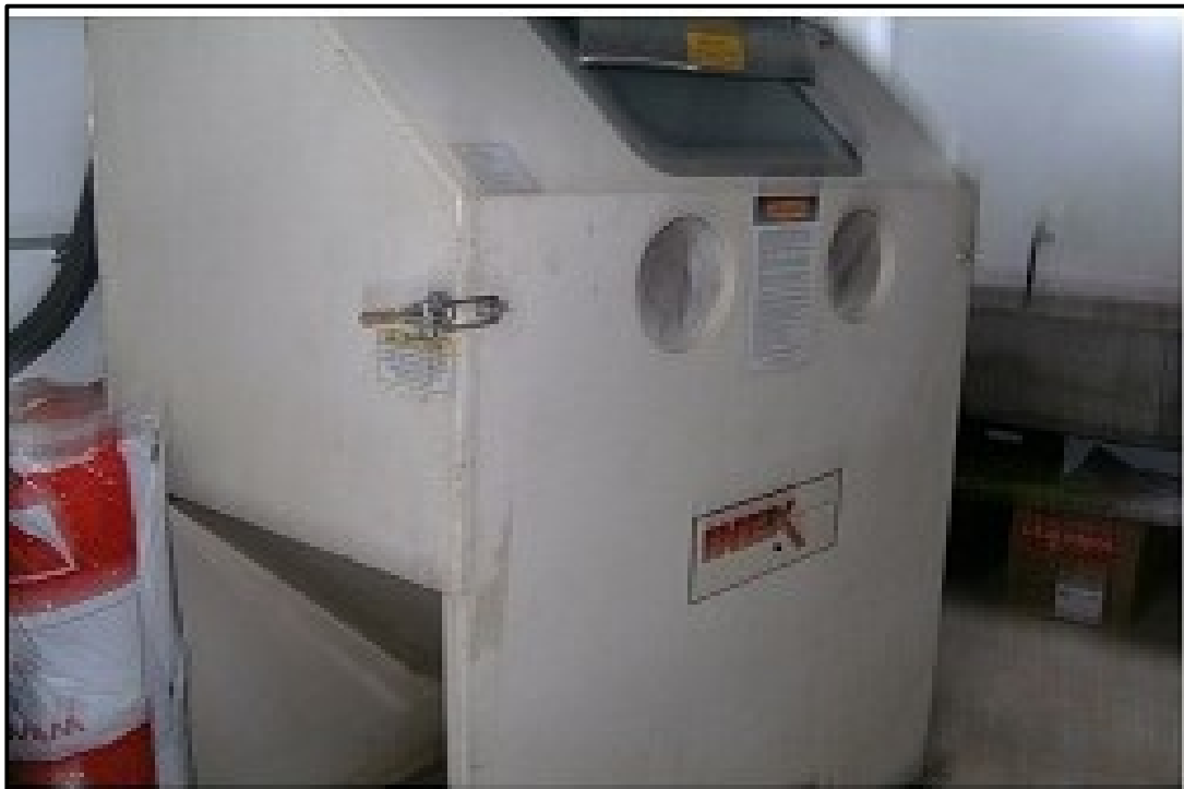
Figura 7.33 Cabina de Sand-blasting a intervenir
