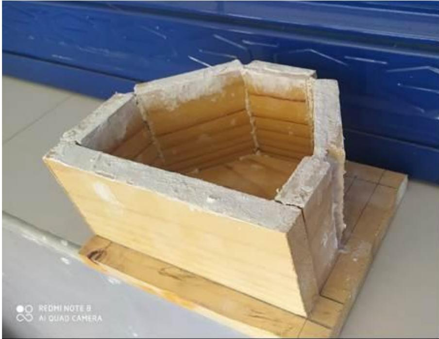
**Figura 32.** Molde madera ladrillo MH
