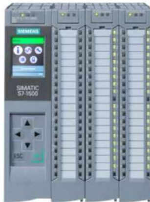
Figura 11 Programmable Logic Controller referencia CPU 1512C-1 PN
