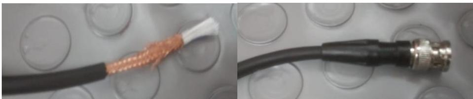
**Figura 3-25.** Cable coaxial y conector macho BNC
