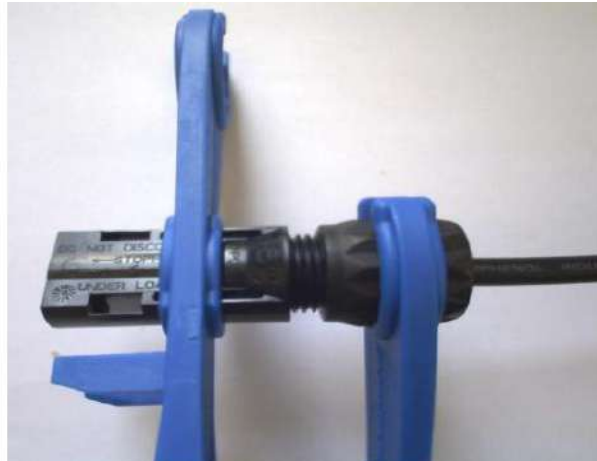
Figure 3-29 Connector body tightening
