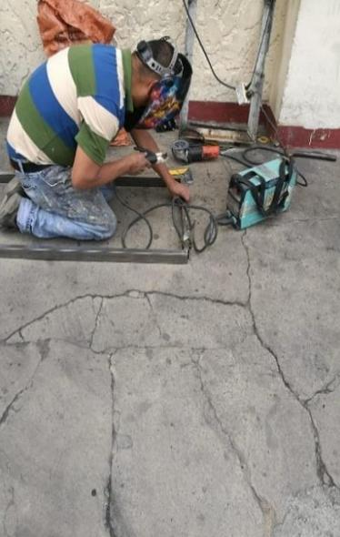
A photograph of a worker in a blue and green striped shirt and a welding mask, kneeling on a concrete floor. He is using a welding torch to weld a metal profile. A blue welding power source is visible on the floor next to him.                                                                                |
