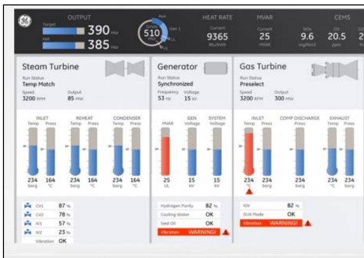
Figura 10. GE Digital HMI/SCADA Cimplicity [44].
