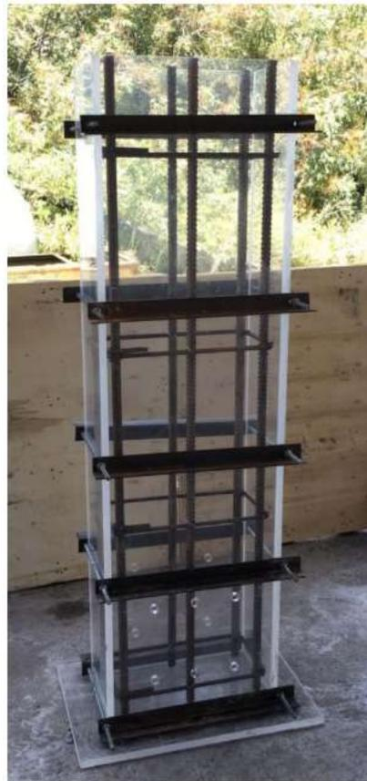
Column containing typical vertical steel of 6 bars Ø20
