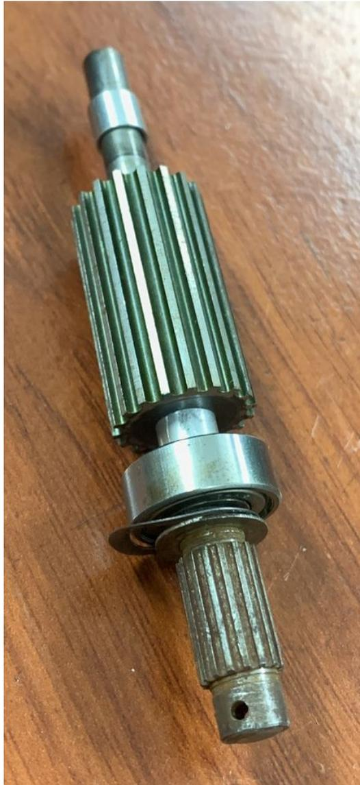
**Figura A.0.8:** . Rotor Motor Emco Compact 5
